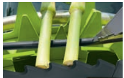
Knives with self-sharpening effect
