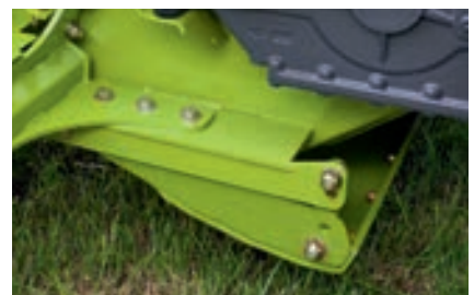
Adjustable skids for the required cutting height
