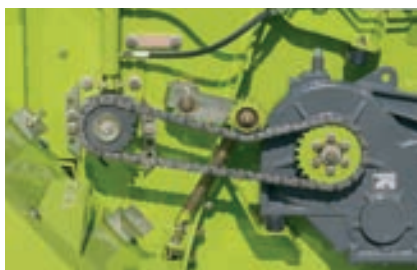
Paddle roller is raised hydraulically
