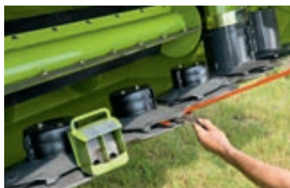
The standard-fit quick knife change dramatically reduces maintenance times.
