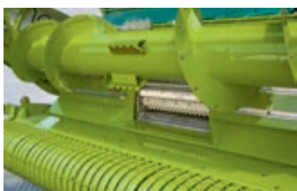
Large auger for high-performance crop flow
