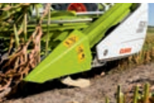
AUTO CONTOUR, ground pressure control with lateral levelling
